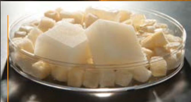
New jelly ice cubes are anti-microbial and prevent cross-contamination, potentially revolutionizing how food is kept cold and shipped fresh without relying on ice or traditional cooling packs.
